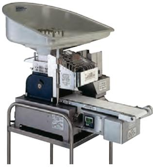
Optional 2' neoprene or wire mesh take away conveyor provides for continuous production. Equipped with a built-in digital programmable counter for accurate patty stacking.
