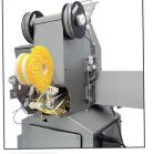
Accessory: automatic loop device with a very easy system to replace the spools.
