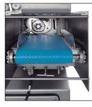
Accessory: automatic conveyor belt to provide an easier release of the products.
